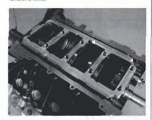
4. Once you've verified the clearance between the main caps and the support plate is good, you can proceed with installing the retaining hardware. There are seven tall metric nuts and two short metric nuts. The short nuts will be used on the rear main studs.
