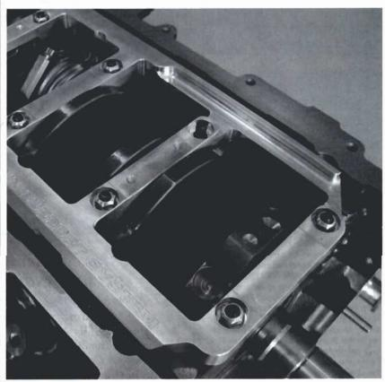
6. With the main support plate secured, Tom carefully rotates the crankshaft, checking each crank throw and connecting rod for proper clearance between themselves and the main support. If there's a tight spot, the main support will have to be removed and clearance made. Do not grind on the main support while it is installed (we hope this is common sense).
