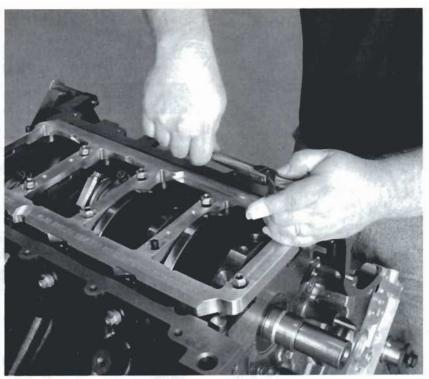
5. Tom Naegle of D.S.S. grabbed the tools to help us with the installation. Tom tightens the retaining hardware so he can check for any interference with the reciprocating assembly.
