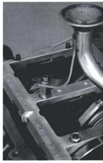
11. Sometimes, the pickup tube bracket will need a light twist to align the hole in it with the pump spacer. Do this gently. Once the mounting bracket and pickup spacer are in alignment, the retaining bolt can be reinstalled as shown.
