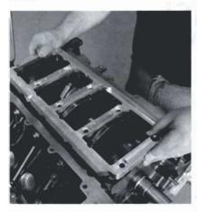
3. The main support simply lies over the longer ARP studs. Check the clearance between the main caps and the support plate—they should not be touching. Clearance of the main support is needed to ensure this.
