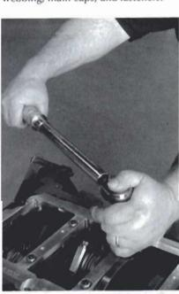
7. Once everything checks out, Tom breaks out the torque wrench and sets the torque on the metric retaining nuts to 30 lb-ft. Notice if you add up the nuts we mentioned earlier, the total comes to nine. We'll show you the 10th retaining nut shortly.
