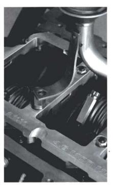
10. Remember that 10th retaining nut we mentioned? It's actually the original oil pickup spacer found on the modular from the factory, though it must be made shorter and the end diameter reduced to clear the main support. The included instructions show the proper dimensions, but it isn't rocket science to modify the spacer.
