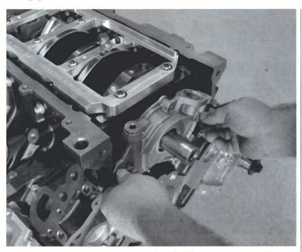
8. Now that the main support is in place, Tom can continue with the final build-up of this modular for one of his customers. The oil pump is driven off the crankshaft on the modulars and slides over the crank snout before being bolted to the block (similar to a transmission front pump).
