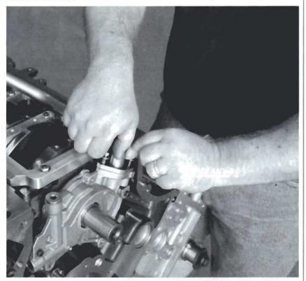
9. The pickup tube on a high-volume oil pump requires a bit of modification before making its way back to the crankcase area of the modular. The crank scraper must be removed from the pickup tube. You can cut this scraper off with a cutoff wheel or hacksaw, but be sure not to cut into the pickup tube. Also, don't forget the O-ring between the pickup tube and the oil pump.
