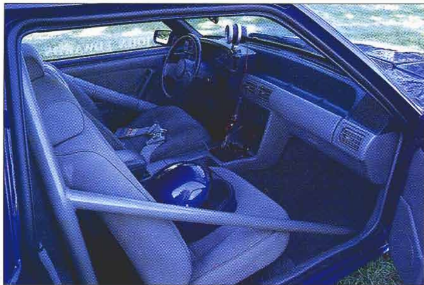
Hey, where's the police radio, the shotgun, the radar, the computer? This officer's office can't be loaded down with all that stuff. An S&W roll bar, Auto Meter tach, a Hurst shifter and RJS safety harnesses are all Edwards needs.
