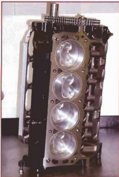
This is the finished short-block with main support installed.
