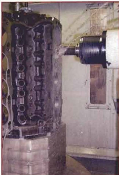
The CNC program machines an offset cylinder chamfer for a 4.100 bore. This 60-degree offset chamfer unshrouds intake and exhaust valves, similar to the Boss 302 and 351 Cleveland. Most aftermarket heads are 4.100 bore, as are the head gaskets. A 4.030 bore block without this chamfer leaves a wall for air and fuel to get around on the side of the valve. This subtle machine operation is one of the horsepower enhancements available with a fully CNC-blueprinted block.
