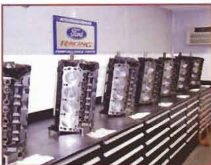
Each DSS engine is assembled in a climate-controlled clean room to prevent contamination of the motor's internals. This isn't exactly your cousin's backyard shed we're talking about here. DSS not only sells to enthusiasts, but it services hardcore racers who demand even more from their engines.
