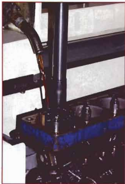
The cylinder is bored .025 over, leaving .005 to hone with torque plates.
