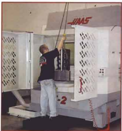
The Haas Horizontal Machining center was purchased and fixtured to blueprint engine blocks. Its size, accuracy and four-axis capability make machining on any part of the block possible. All fixturing is done off of the main saddles (not the oil pan rail like some other machines) with the end result being a very accurate, rigid, repeatable fixture that allows for proper machining and squaring of the block.
