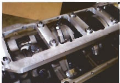
Note how the DSS main support girdle is cleared for the connecting rods. All bolts are triple checked to ensure your motor is ready to go when you receive it.
