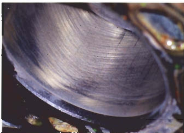
Despite the mileage, oil of the cylinders still bore the original cross-hatch marks.
