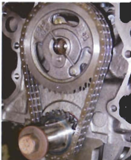
We had only logged 140-some miles on the Comp Cams double roller timing chain that we installed when we swapped the Brodix heads on, so we reused it.
