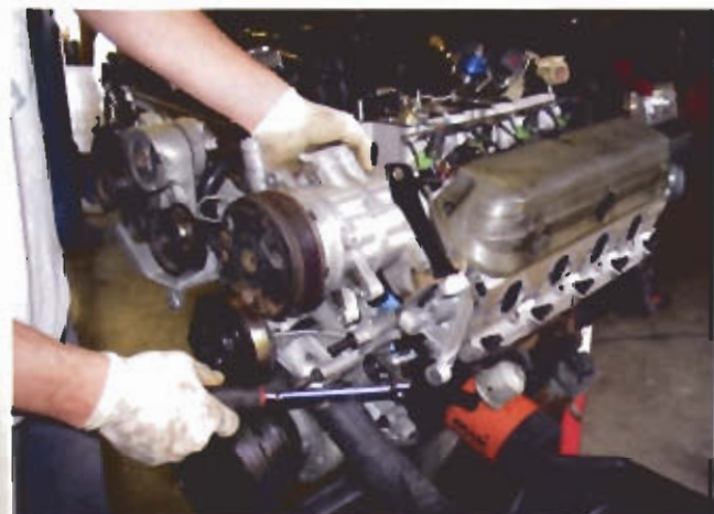
Glenn disassembles the 5.0-liter, as we will be reusing many of the existing parts including the cylinder heads, intake manifold and timing chain.
