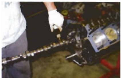
For our camshaft, we chose a Comp Cams XE274HR grind. This exact cam (PN 35-518-8, $234.95) was used with our Brodix heads in our "Ultimate Guide to Cylinder Heads" (MM&F November 2003) and produced 434 hp in a naturally aspirated 331-inch engine.
