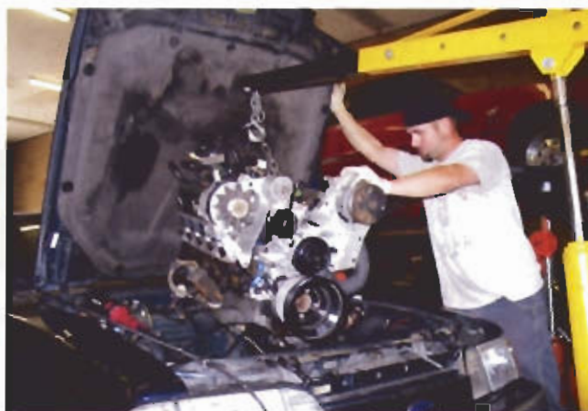
Before we start bolting on the ports though, the old motor has to come out. It has served us well for its 143,000 miles and was good for 473 rwhp.
