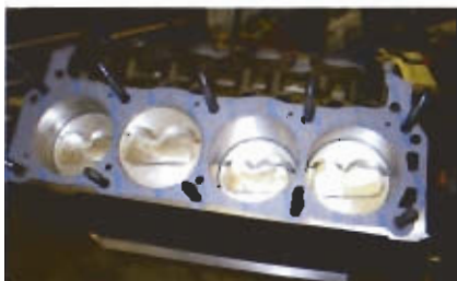
We also reused our ARP head studs. For head gaskets, we chose the factory graphite pieces. According to Tom Naegele at DSS, they've seen great power had with graphite or Cometic gaskets. Obviously the SuperPro Bullet's straight deck and O-rings help keep everything in its place.
