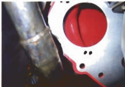
Long-tube headers generally have a clearance problem with the bellhousing, which is one reason why most race headers are fabricated. Cutting the bell housing technically negates its SFI rating, but we're more worried about our ankles, not the regulations. Glenn used a plasma cutter to notch out the metal on the passenger side and then ground down the rough edges for a finished look.
