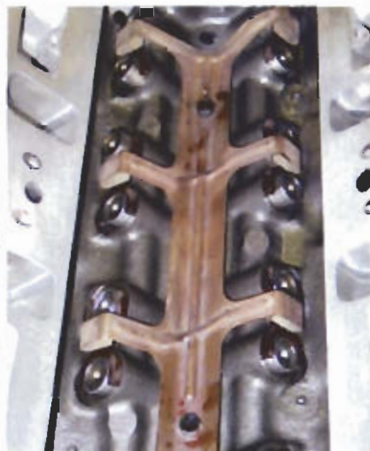
Considering the mileage, the stock roller lifters had served their duty well, and despite not showing any real signs of wear, the factory pieces were traded in for a fresh set from Comp Cams (PN 851-16). The lifter cage was cleaned and bolted to the new engine.
