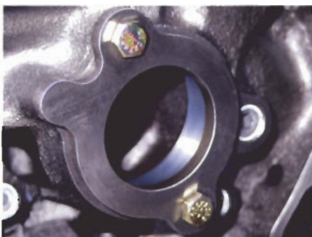
DSS includes a new cam plate, as well as dowel pins for the cylinder heads.
