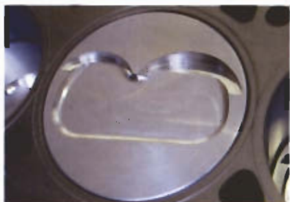
Here you can see the DSS reverse dome low-compression piston. We opted for the O-ringed block to make sure we keep the cylinder pressure where it needs to be.
