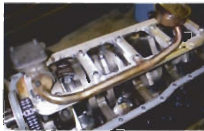
We ordered a new stock oil pump as it offers plenty of petroleum for our pony's powerplant. The stock pickup was cleaned and reused.
