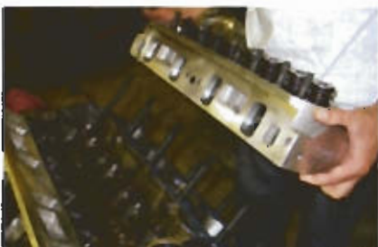
The Brodix M2 ST5.0R heads were installed and torqued to 80 ft-lb. We let them sit for 30 minutes and then backed them off and retorqued them to 85 ft-lb. to make sure there was no more stretch.
