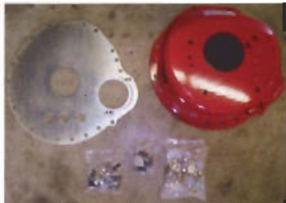
Something else we thought we should upgrade was the bellhousing. Knowing that our pony has some clutch drops in its near future, we heaved the stock aluminum bell housing in favor of this SFI-approved racing piece from Lakewood. Retail price for this steel scattershield (PN LKW 15203) is $339.90. We're fairly sure our Clutchmasters aluminum flywheel will hold together, but it certainly won't hurt to have one.
